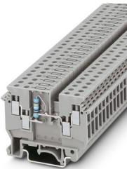
Component terminal block, nom. voltage: 630 V, nominal current: 32 A, number of connections: 4, connection method: Screw connection, Rated cross section: 4 mm<sup>2</sup>, 1 level, cross section: 0.2 mm<sup>2</sup> - 6 mm<sup>2</sup>, mounting type: NS 35/7,5, NS 35/15, NS 32, color: gray
