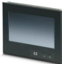
Maritime-Panel PC, 17.8 cm / 7"-TFT display (Analog resistive (GFG)), 800 x 480 pixel(s) (WVGA), 262144 colors, Intel® Atom™ E680T 1.6 GHz, 4x USB Host 2.0, 1x COM (RS-232), 1x COM (RS-232/485), 2x Ethernet (10/100/1000 Mbps), RJ45, Windows® Embedded Standard 7, TSvisIT, DualCAN.
