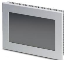
Rugged-Touch panel, 17.8 cm / 7"-TFT display (Analog resistive (GFG)), 800 x 480 pixel(s) (WVGA), 16.7 million colors, Arm® Cortex®-A8, 1000 MHz, 2x USB Host 2.0, 1x COM (RS-232), 1x COM (RS-232/485), 1 x Ethernet (10/100 Mbps), RJ45, Windows® Embedded Compact 7, Open platform, DualCAN.
