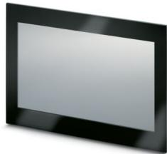
IP65-rated, 21.5-inch, flat panel LCD monitor with projected capacitive touch screen
