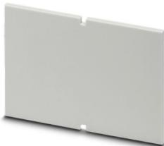
Side panel for use with housing half shells 125 x 87 mm in size; panel thickness: 2 mm; total height of housing: 47 mm; material: polycarbonate; color: light gray similar to RAL 7035
