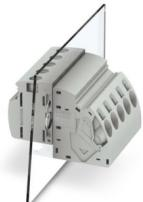
Panel feed-through terminal block, connection method: Push-in spring connection, Screw connection with tension sleeve, number of positions: 1, load current: 76 A, cross section: 1.5 mm<sup>2</sup> - 16 mm<sup>2</sup>, connection direction of the conductor to plug-in direction: 45 °, width: 12 mm, color: gray
