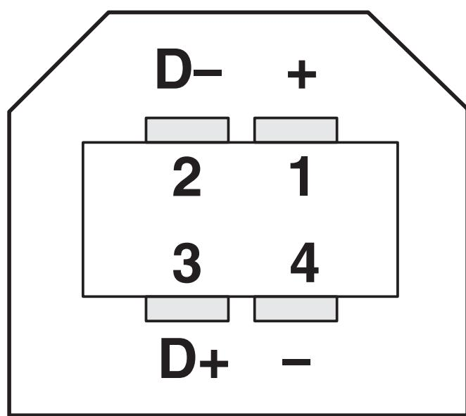
Plug pin assignment plug USB, type B
