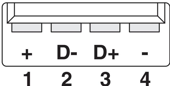
Pin assignment plug USB, type A
