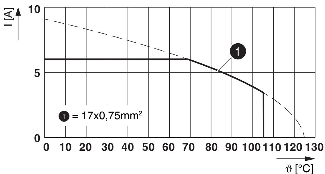
$I$  = current strength,  $\vartheta$  = ambient temperature,  $17 \times 6$  A
