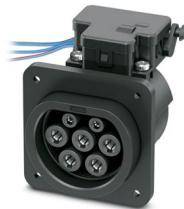
CHARX connect, Type 2, Infrastructure charging socket, 20 A, 480 V AC, length: 0.5 m, locking actuator: 12 V, 4-pos., Rear panel mounting, additional splash protection at the rear with single-core wire seals, for charging electric vehicles (EV) with alternating current (AC), PHOENIX CONTACT logo, IEC 62196-2
