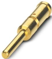
Crimp contact, Pin, turned, contact diameter: 2 mm, connection cross section: 0.25 mm<sup>2</sup> ... 1 mm<sup>2</sup>, contact material: CuZn, Alternative product in accordance with RoHS II without Exemption 6c (Pb < 0.1 %) item no.: 1244464
