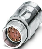
M23, Coupler connector, series: CA, straight, shielded: yes, for standard and SPEEDCON interlock, No. of pos.: 12, Direction of rotation: Standard, contact connection type: Socket, Crimp connection, cable diameter range: 10 mm ... 14.5 mm, coding: N
