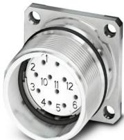
M23, Device connector front mounting, series: CA, straight, shielded: yes, for standard and SPEEDCON interlock, No. of pos.: 12, Direction of rotation: Standard, contact connection type: Socket, Solder connection, Flat gasket, flange dimensions: 25 mm x 25 mm, coding: N. This product is in the process of being discontinued. This product must no longer be considered for new projects. Please contact your sales representative for alternatives.
