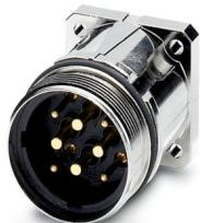
Device connector front mounting, straight, for standard and SPEEDCON interlock, M40, number of positions: 2+3+PE, contact connection type: Pin, Axial O-ring, shielded: yes, flange dimensions: 40 mm x 40 mm, number of positions: 6, connection method: Crimp connection, series: SM, this item is expected to be lead-free from Q2 2026 in accordance with RoHS II without exception 6c (Pb < 0.1%), a lead-free alternative is possible on request in advance
