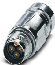
Coupler connector, straight, for standard and SPEEDCON interlock, M17, number of positions: 7+PE, contact connection type: Socket, shielded: yes, degree of protection: IP67, cable diameter range: 8 mm ... 10 mm, number of positions: 8, connection method: Crimp connection, series: ST. This product is in the process of being discontinued. This product must no longer be considered for new projects. Please contact your sales representative for alternatives.
