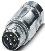
Coupler connector, straight, for standard and SPEEDCON interlock, M17, number of positions: 5+PE, contact connection type: Pin, shielded: yes, degree of protection: IP67, cable diameter range: 5 mm ... 8 mm, number of positions: 6, connection method: Crimp connection, series: ST, This product is in the process of being discontinued. This product must no longer be considered for new projects. Please contact your sales representative for alternatives.
