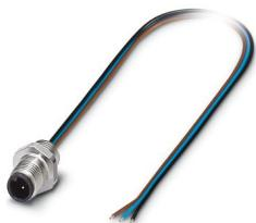
Device connector front mounting, 3-position, Pin, straight, M5, A-coding, Individual wires, cable length: 0.5 m, 0.14 mm<sup>2</sup>, TPE litz wire
