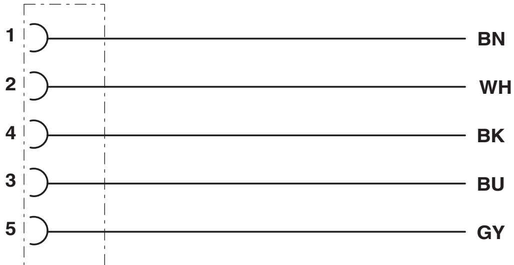
Contact assignment of the M12 socket
