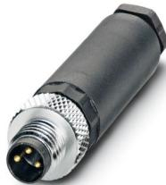
Connector, Universal, 3-position, Plug straight M8, coding: A, Screw connection, knurl material: Brass, nickel-plated, external cable diameter 3.5 mm ... 5 mm
