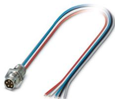
Device connector front mounting, DeviceNet™, 5-position, Pin, straight, M8, Individual wires, cable length: 0.5 m, 0.25 mm<sup>2</sup>, PVC litz wire
