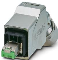
RJ45 connector, degree of protection: IP65/IP67, number of positions: 8, 1 Gbps, CAT5, material: Metal, connection method: IDC fast connection, connection cross section: AWG 26- 24, cable outlet: angled, Ethernet
