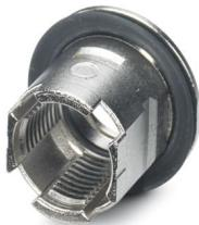
M12 threaded sleeve with tolerance-compensating function, for straight, THR solderable M12 socket contact inserts. Suitable for 1.7 mm ... 2.5 mm thick front plates.
