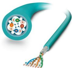
By the meter, Data cable, Ethernet CAT5 (1 Gbps), shielded, PUR halogen-free, water blue RAL 5021, 8-wire (4x2xAWG26/19, S/UTP), color single wire: white/blue-blue, white/orange-orange, white/green-green, white/brown-brown, cable length: 100 m
