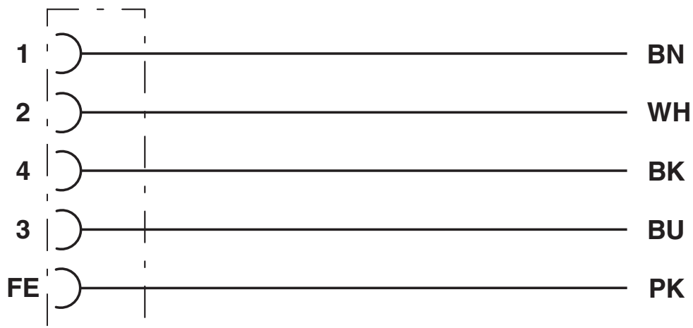
Contact assignment of the M12 socket
