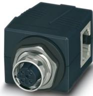
Control cabinet feed-through, M12, 4-pos., D-coded to RJ45 socket, socket entry: 90°, IP65/IP67
