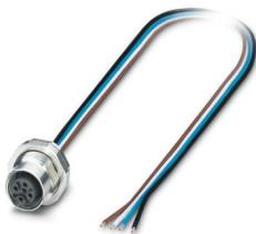
Device connector rear mounting, Universal, 4-position, Socket, straight, M12-Standard, A-coding, on free cable end, Individual wires, cable length: 0.5 m, 0.34 mm<sup>2</sup>, TPE litz wire, potted
