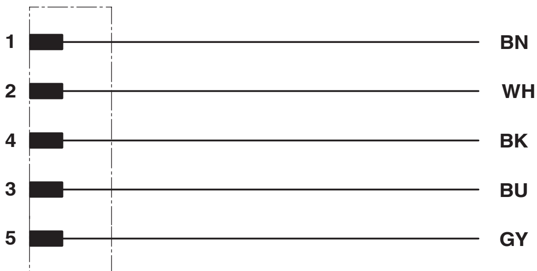
Contact assignment of the M8 plug
