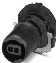
SPE PCB connector, design: SPE, degree of protection: IP65/IP67, number of positions: 2, material: LCP, connection method: THR solder connection, cable outlet: straight, color: black, Single Pair Ethernet
