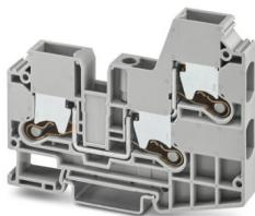
Feed-through terminal block, nom. voltage: 1000 V, nominal current: 57 A, number of connections: 3, number of positions: 1, connection method: Push-X-connection, Rated cross section: 10 mm<sup>2</sup>, cross section: 1.5 mm<sup>2</sup> - 16 mm<sup>2</sup>, mounting type: NS 35/7,5, NS 35/15, color: gray
