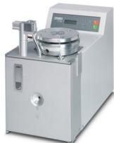
Automatic stripping and crimping device, input voltage 100 V ... 240 V, electro-pneumatic, for loose ferrules with insulating collar, 4 mm<sup>2</sup>, 6 mm<sup>2</sup>, and 10 mm<sup>2</sup>, without conversion kit
