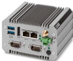
IP30-rated fanless industrial box PC (BPC) with energy-efficient Intel® Celeron® N3350 processor with 32 GB eMMC mass storage, 128 GB M.2 SSD, 2x COM ports, Windows 10 Enterprise 2019 LTSC operating system, Wi-Fi, and a Trusted Platform Module (TPM)
