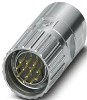
M23, Cable connector, series: M23 PRO, straight, shielded: yes, Screw locking mechanism, No. of pos.: 12, Direction of rotation: Counter direction, contact connection type: Pin, Crimp connection, cable diameter range: 4 mm ... 8.5 mm, coding: N, Item is lead-free in accordance with RoHS II without Exemption 6c (Pb < 0.1 %)
