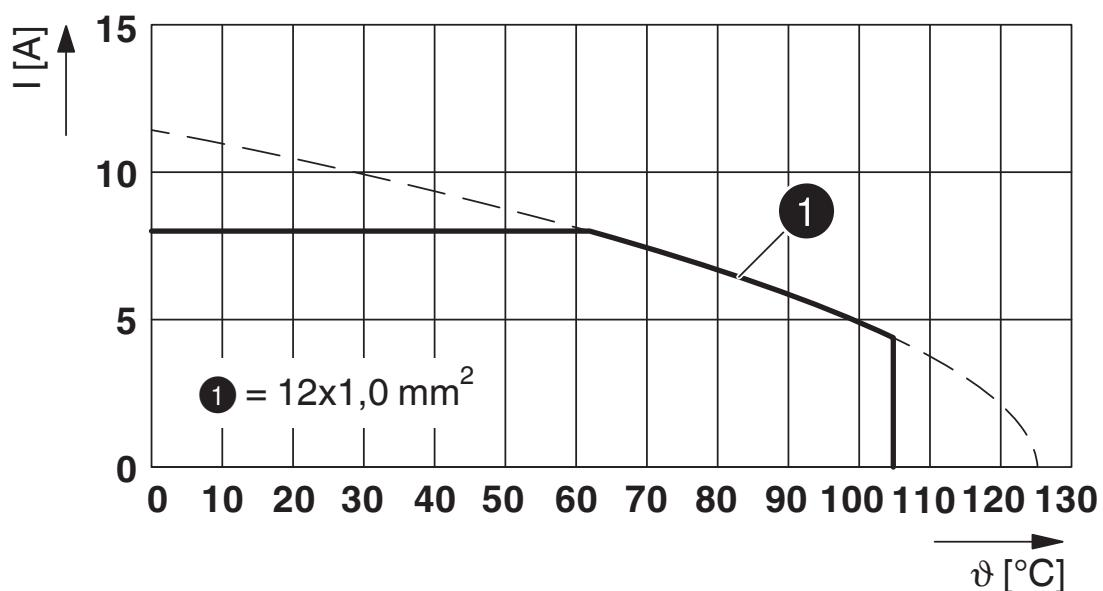
$I$  = current strength,  $\vartheta$  = ambient temperature,  $12 \times 8 \text{ A}$
