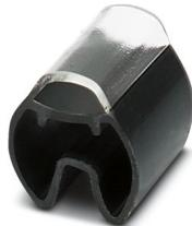
Conductor marker carrier, transparent/black, unmarked, cable diameter range: 4 ... 7 mm, mounting type: slide-on, text field height: 4 mm, text field width: 30 mm
