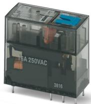
Plug-in miniature relay, with power contact, 1 changeover contact, test button, mechanical switch position indicator, polarity: bipolar, input voltage: 24 V DC
