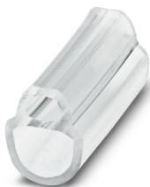
Conductor marker carrier, transparent, unmarked, cable diameter range: 0.6 ... 1.2 mm, mounting type: slide-on, text field height: 4 mm, text field width: 10 mm
