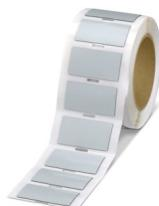
Label, Roll, silver, unmarked, can be labeled with: THERMOMARK E.300 (D)/600 (D), THERMOMARK ROLL 2.0, THERMOMARK ROLL, THERMOMARK ROLL X1, THERMOMARK ROLLMASTER 300/600, THERMOMARK X1.2, mounting type: adhesive, Number of individual labels: 250, text field height: 30 mm, text field width: 60 mm
