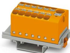
Distribution block, nom. voltage: 800 V, nominal current: 32 A, number of connections: 13, connection method: Push-in connection, Rated cross section: 4 mm<sup>2</sup>, Load contact, cross section: 0.2 mm<sup>2</sup> - 6 mm<sup>2</sup>, Push-in connection, Line contact, Rated cross section: 10 mm<sup>2</sup>, cross section: 0.5 mm<sup>2</sup> - 10 mm<sup>2</sup>, mounting type: NS 35/7,5, NS 35/15, color: orange
