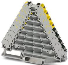
Potential distributors, without actuating push button, nom. voltage: 250 V, nominal current: 17.5 A, connection method: Push-in connection, 1st, 2nd, 3rd, 4th, 5th, 6th, 7th and 8th level, Rated cross section: 1.5 mm<sup>2</sup>, cross section: 0.14 mm<sup>2</sup> - 2.5 mm<sup>2</sup>, mounting: NS 35/7,5, NS 35/15, color: gray, color of connection elements: yellow, black
