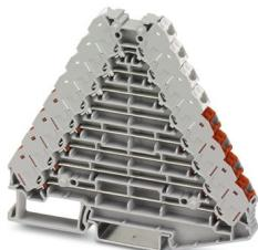
Marshalling panel, without actuating push button, nom. voltage: 250 V, nominal current: 8 A, connection method: Push-in connection, 1st, 2nd, 3rd, 4th, 5th, 6th, 7th and 8th level, Rated cross section: 1.5 mm<sup>2</sup>, cross section: 0.14 mm<sup>2</sup> - 2.5 mm<sup>2</sup>, mounting: NS 35/7,5, NS 35/15, color: gray, color of connection elements: white, red
