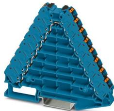
Potential distributors, nom. voltage: 250 V, nominal current: 17.5 A, connection method: Push-in connection, 1st, 2nd, 3rd, 4th, 5th, 6th, 7th and 8th level, Rated cross section: 1.5 mm<sup>2</sup>, cross section: 0.14 mm<sup>2</sup> - 2.5 mm<sup>2</sup>, mounting: NS 35/7,5, NS 35/15, color: blue, color of connection elements: black
