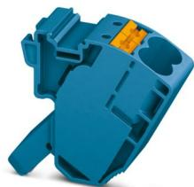
Pick-off terminal block, nom. voltage: 1500 V, nominal current: 57 A, number of connections: 2, connection method: Push-in connection, Rated cross section: 10 mm<sup>2</sup>, 1 level, cross section: 0.5 mm<sup>2</sup> - 16 mm<sup>2</sup>, mounting type: on base element, color: blue
