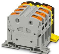
High-current terminal block, Blocked, nom. voltage: 1000 V, nominal current: 232 A, number of connections: 8, number of positions: 4, connection method: PowerTurn connection, cross section: 25 mm<sup>2</sup> - 95 mm<sup>2</sup>, mounting type: direct screw connection, color: gray/black-yellow
