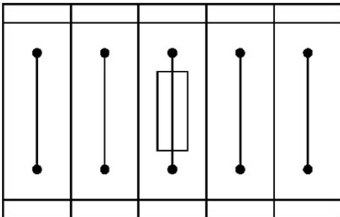
Fuse terminal block in single arrangement,
