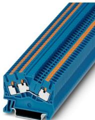
Feed-through terminal block, nom. voltage: 800 V, nominal current: 24 A, number of connections: 3, connection method: Push-in connection, Rated cross section: 2.5 mm<sup>2</sup>, 1 level, cross section: 0.14 mm<sup>2</sup> - 4 mm<sup>2</sup>, mounting type: NS 35/7,5, NS 35/15, color: blue
