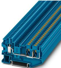
Feed-through terminal block, nom. voltage: 800 V, nominal current: 32 A, connection method: Push-in connection, Rated cross section: 4 mm<sup>2</sup>, cross section: 0.2 mm<sup>2</sup> - 6 mm<sup>2</sup>, connection method: Screw connection, Rated cross section: 4 mm<sup>2</sup>, cross section: 0.14 mm<sup>2</sup> - 6 mm<sup>2</sup>, mounting: NS 35/7,5, NS 35/15, color: blue
