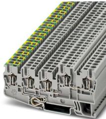
Installation protective conductor terminal block, nom. voltage: 250 V, nominal current: 18 A, number of connections: 5, connection method: Spring-cage connection, Rated cross section: 2.5 mm<sup>2</sup>, cross section: 0.08 mm<sup>2</sup> - 4 mm<sup>2</sup>, mounting type: NS 35/7,5, NS 35/15, color: gray
