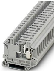
Disconnect terminal block, Current and voltage are determined by the plug used., With test socket screws for insertion of test plugs, nom. voltage: 500 V, nominal current: 20 A, connection method: Screw connection, Rated cross section: 2.5 mm<sup>2</sup>, cross section: 0.2 mm<sup>2</sup> - 10 mm<sup>2</sup>, mounting: NS 35/7,5, NS 35/15, color: gray
