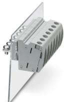
Panel feed-through terminal block, connection method: Screw connection with tension sleeve, Cable lug connection, number of positions: 1, load current: 76 A, cross section: 6 mm<sup>2</sup> - 25 mm<sup>2</sup>, connection direction of the conductor to plug-in direction: 0 °, width: 12.1 mm, color: gray. Item with lateral securing pin
