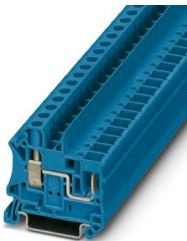
Feed-through terminal block, nom. voltage: 1000 V, nominal current: 41 A, number of connections: 2, connection method: Screw/plug-in connection, Rated cross section: 6 mm<sup>2</sup>, cross section: 0.2 mm<sup>2</sup> - 10 mm<sup>2</sup>, mounting type: NS 35/7,5, NS 35/15, color: blue
