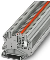
Knife-disconnect terminal block, with actuation latch, nom. voltage: 500 V, nominal current: 20 A, connection method: Screw connection, Rated cross section: 2.5 mm<sup>2</sup>, cross section: 0.14 mm<sup>2</sup> - 6 mm<sup>2</sup>, mounting: NS 35/7,5, NS 35/15, color: gray
