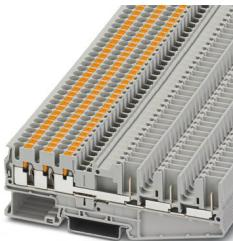
Feed-through terminal block, nom. voltage: 500 V, nominal current: 24 A, number of connections: 6, connection method: Push-in / plug connection, Rated cross section: 2.5 mm<sup>2</sup>, 1st, 2nd and 3rd level, cross section: 0.14 mm<sup>2</sup> - 4 mm<sup>2</sup>, mounting type: NS 35/7,5, NS 35/15, color: gray
